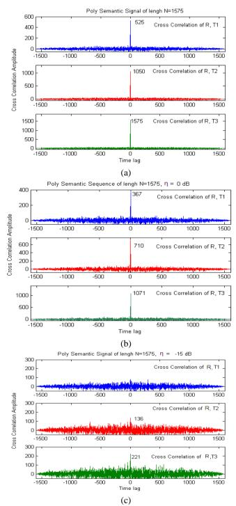
Fig. 8 Coincidence detection of the poly-semantic sequence at length N=1575 (a) when no noise (b)  $\eta = 0$  dB and (c)  $\eta = -15$  dB
