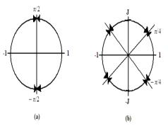
Fig. 1 Range of phase shift without bit errors (a) for bi-phase sequences (M=2) (b) poly-phase sequences with M = 4.
