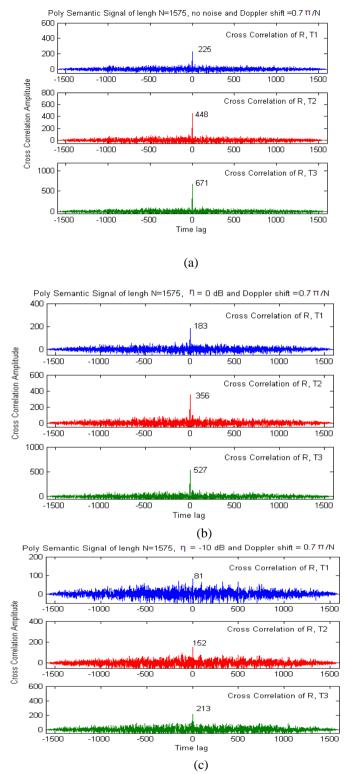
Fig. 9 Coincidence detection of the poly-semantic sequence at length N=1575 (a) when no noise, Doppler shift  $0.7\pi/N$ , (b)  $\eta = 0 \text{ dB}$ , Doppler shift  $0..7\pi/N$  and (c)  $\eta = -10 \text{ dB}$ , Doppler shift  $0..7\pi/N$
