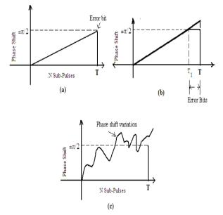
Fig. 2 Doppler phase shift on received bi-phase sequences (a) when phase shift is equal to  $\pm \pi/2$  (b) when phase shift is greater than  $\pm \pi/2$  (c) when additive noise is added along with Doppler phase shift.
