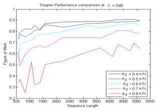
Fig. 6 Noise and Doppler performance of poly-semantic sequences at different Doppler phase shifts ( $\phi_d$ ) and fixed  $\eta$  of 0 dB.
